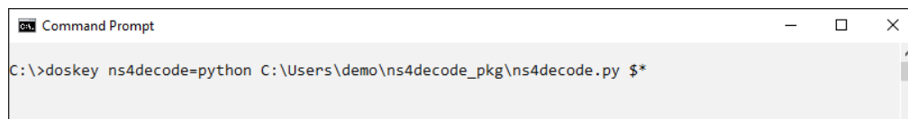
Figure 7.3: Example of the full abbreviation-creating command for Windows. The path to ns4decode on your computer will be different.
